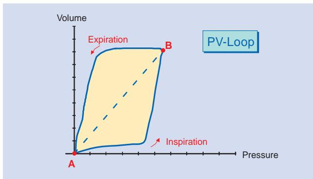
Assumptions cannot be made on the basis of this loop about the course of lung compliance. When the breathing gas flow is equal to zero at the end of inspiration, however, the steepness of a line drawn between the start of inspiration (A) and the point at the end of inspiration (B) does represent a measure of dynamic compliance. This presupposes, however, that flow equals zero both at the end of inspiration and at the end of expiration.
