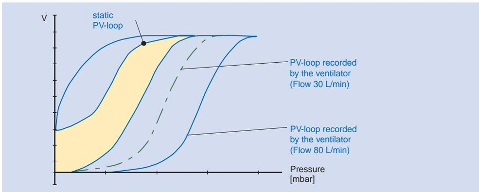
Since ventilators open the exhalation valve either to ambient pressure or set PEEP at the beginning of expiration, the pressure displayed by the PV loop also falls almost immediately to this value.
