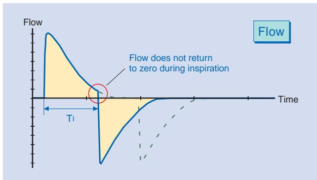
**The flow curve in the case of insufficient inspiration time**
