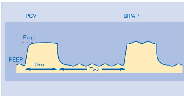
Pressure-time diagramm for pressure controlled ventilation.
