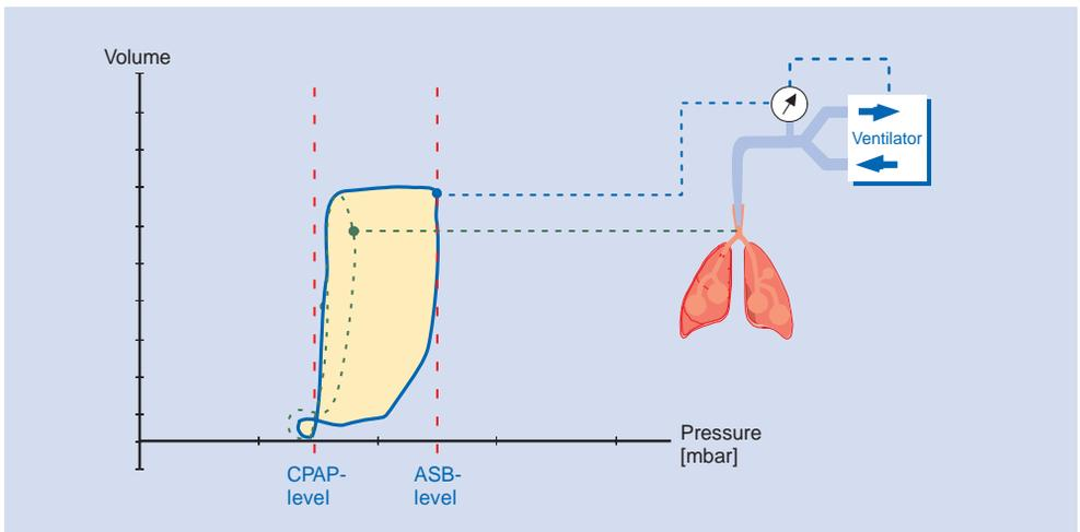
If the inspiratory branch of the loop lies exactly on the vertical line of the CPAP set value, the tube resistance will only just be compensated for. If the inspiratory branch lies to the right of the CPAP line then support is provided above and beyond merely compensating for the tube resistance, thus compensating for possible pathological resistances in the lower airways. If the
