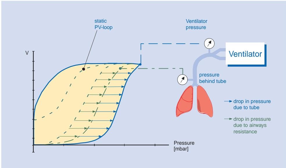
For this reason the PV loop does not give an accurate picture of the course of compliance. The greater the inspiratory breathing gas flow the greater the additional pressure gradient and thus the degree of inaccuracy.
