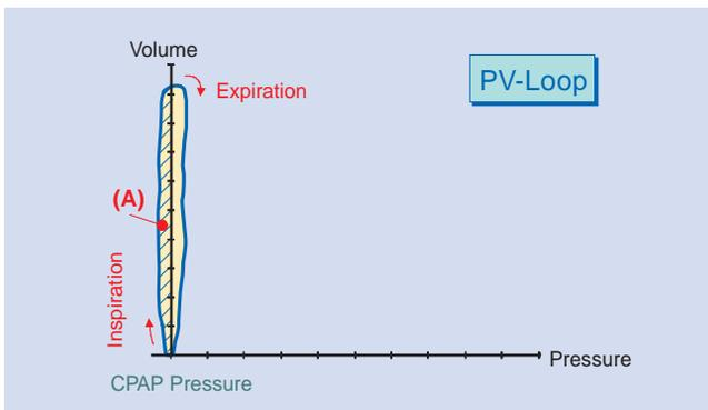
The ventilator always tries to supply the patient with enough breathing gas to ensure that the set CPAP pressure is maintained at a constant level, although a slight negative deviation is inevitable. The area to the left of an imaginary vertical axis (A) at the set CPAP pressure is thus a measure of the patient's efforts to combat the inspiratory resistances of the ventilator.
