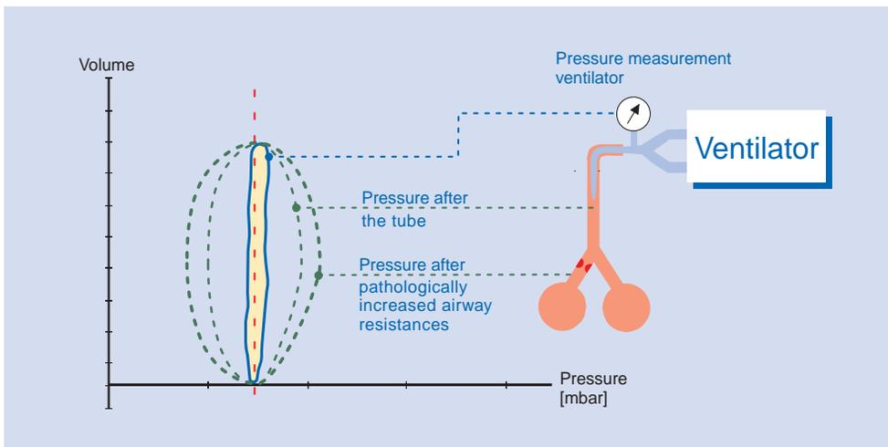
The smaller the tube diameter the more the patient has to work to combat the tube's resistance [4], a fact which is shown by the different area covered by the loops recorded after the tube.
