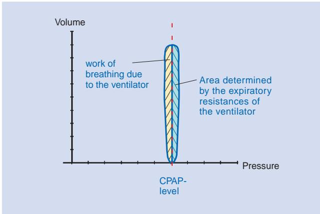
The belief that a narrow PV loop is synonymous with less work of breathing for the patient is not correct in every case.
