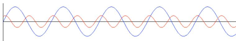
**Fig. 3** Two sine waves of differing frequency, amplitude and phase
