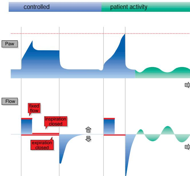
mandatory phase activate high airway pressure alarms. The freedom for the patient to cough freely and clear his own secretions during volume controlled modes is usually suppressed. In any situation AutoFlow® always provides safety and lower pressures compared to normal volume controlled modes.
