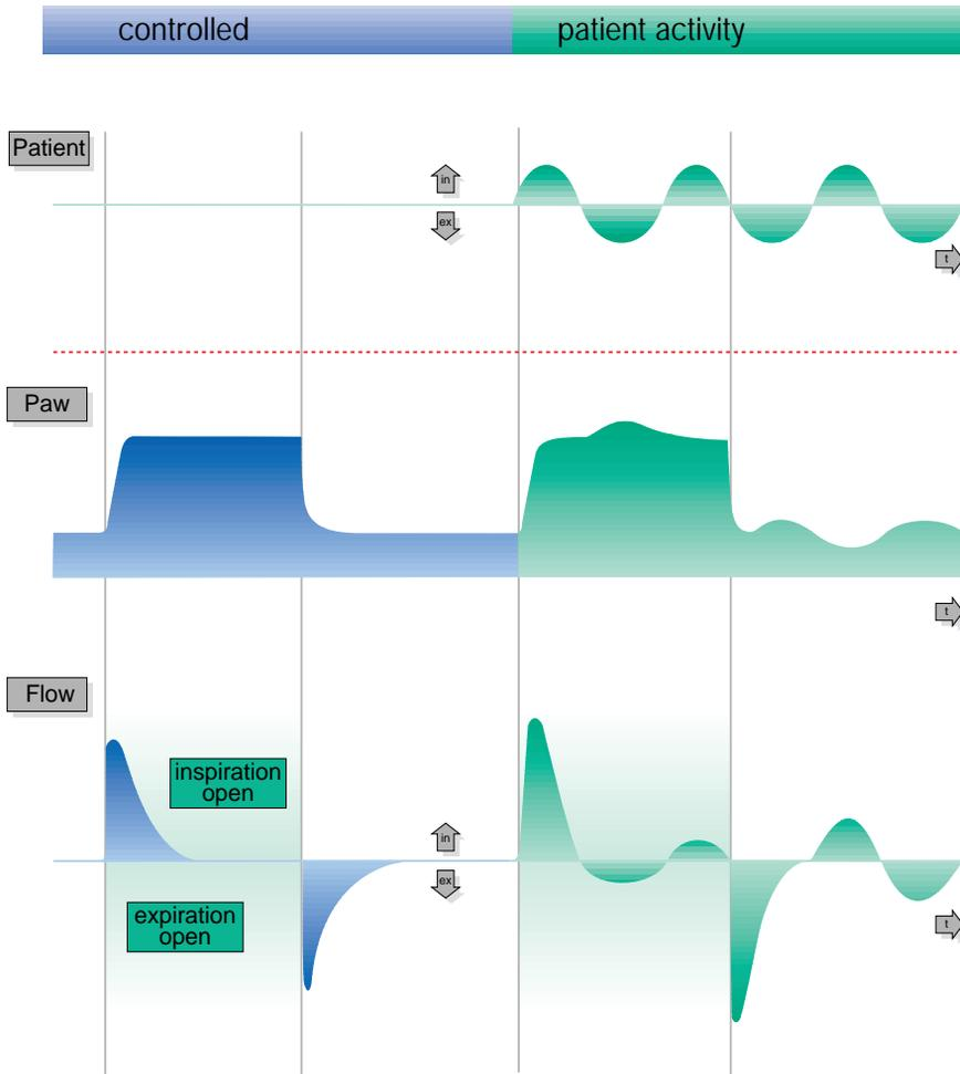
AutoFlow® responds like a CPAP system with CPAP value set to  $P_{\text{insp}}$ . Whenever the patient tries to inhale more volume the demand valve will deliver more flow, whenever he wants to exhale the expiration valve will allow expiratory flow while the pressure/PEEP level is kept constant. The graphs above illustrate this.
