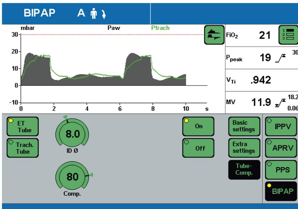
The length of the tube has no significant bearing on the tube resistance even in the case of shortened tubes, and consequently does not need to be entered.
