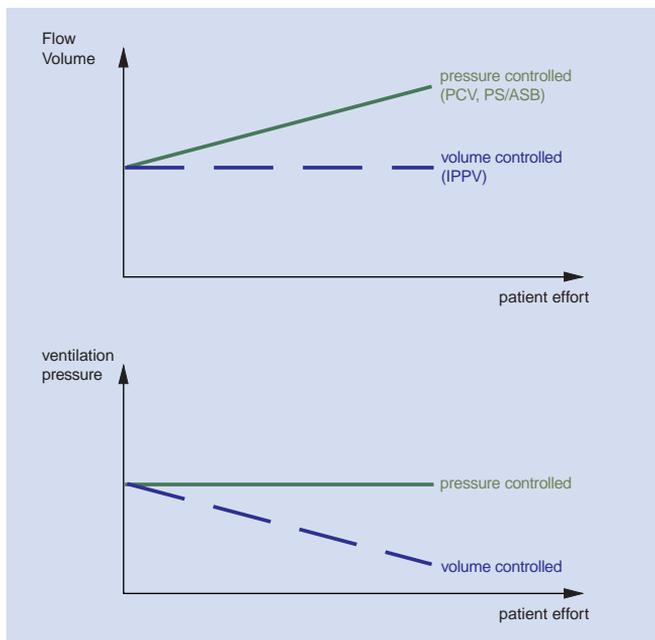
Whereas the classical volume-controlled modes do not show any reaction with regard to flow and volume, the pressure-controlled modes react by increasing flow and volume. Important in this context is only the basic correlation; the starting values shown in the diagrams for zero inspiratory effort are chosen at random and of course depend exclusively on the ventilator settings.
