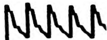
This is a trace from an *underdamped* IABP system. The damping co-efficient is  $<0.7$ . This system will be quick to respond but will tend to overshoot and oscillate around its resting point, over-reading SBP and under-reading DBP.
